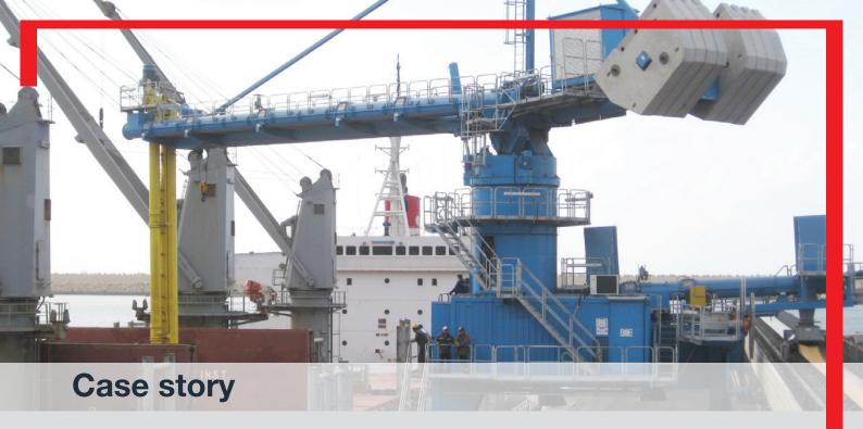
These unloaders discharge the grain to a jetty belt conveyor behind the units, however, the unloaders are also equipped with two discharge bellows placed beneath the main beam to allow direct discharge to trucks, when needed.
