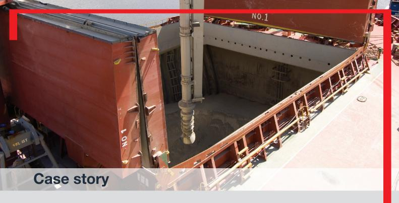
The Siwertell ship unloader is part of a cement handling terminal in Houston, Texas, USA, which includes unloading and storage in silos of 100,000t in total. With low costs for maintenance and power consumption, this heavy-duty unloader is exceptionally suitable for the terminal's high yearly throughput.
