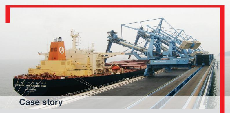
The material transport is, thanks to a specially designed arrangement, completely enclosed and covered, from the ship's hold to the gantry conveyor, and onwards to the quay conveyor as well as to the storage facility. This way, dust emission and spillage is eliminated, which makes the installation highly environmentfriendly.
